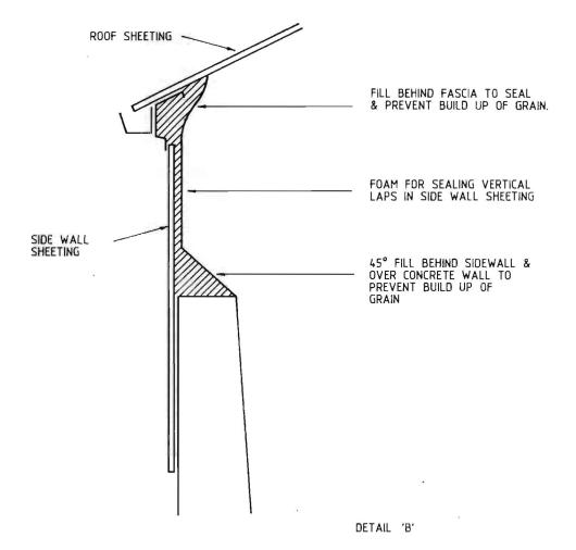
FIG. 5. DETAIL OF USE OF FOAM POLYURETHANE TO FILL WALL - TO - ROOF JOIN IN A STEEL - CLAD HORIZONTAL STORAGE.
