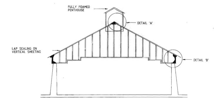
FIG. 3. END ELEVATION OF A TYPICAL HORIZONTAL OR SHED-TYPE STORAGE SHOWING REGIONS WHERE POLYURETHANE FOAM IS USED.
