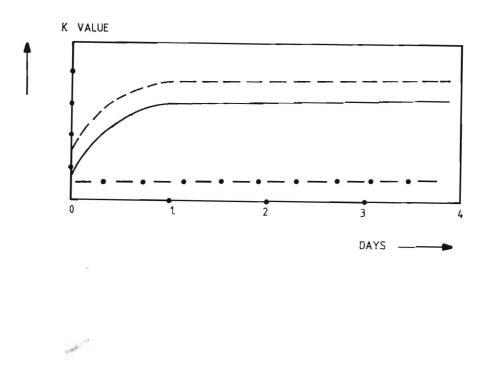
FIG. 2. CHANGE IN THERMAL CONDUCTIVITY WITH TIME FOR POLYURETHANE FOAM WITH DIFFUSION - TIGHT FACINGS : ' WITH NORMAL SURFACE SKIN WITH CUT SURFACE
